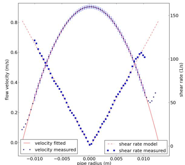
Figure 1: Velocity profile measured and fitted by a Newtonian model, and the shear rate associated for sunflower oil with a Doppler angle of 35°, transducer on left side.
