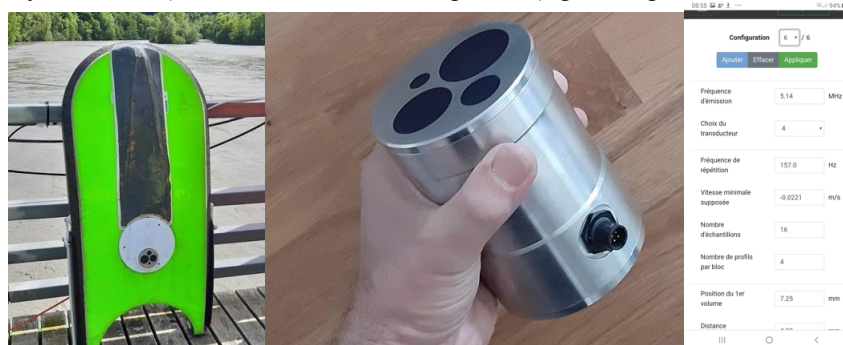
Fig. 1. From left to right : the UB-SediFlow on a floating board, the acoustic module and the user interface
