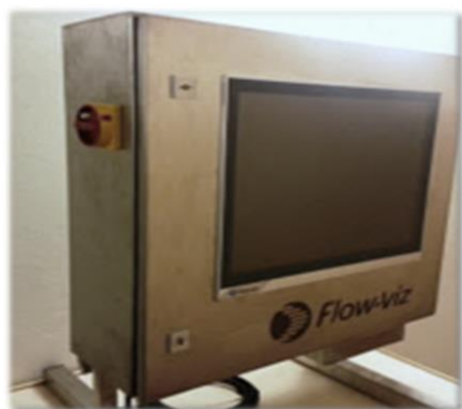
Figure 1: The Flow-Viz™ operator's panel featuring the electronics, main Industrial PC unit, sensor block and multi-touch monitor.
