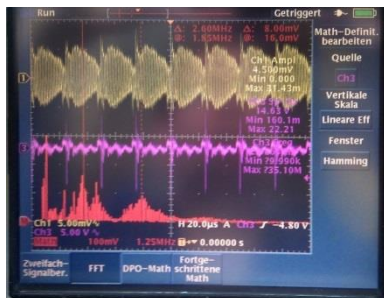
Figure 4: Oscilloscope signals of a supply lines (SL). Top (yellow): CH1, magnetic stray field, picked up with an air coil. – Middle (purple): CH3 AC measurement of SL. – Bottom (red): Fourier transform of CH3, with a clear-cut minimum at 3.5 MHz and a peak at 4 MHz
