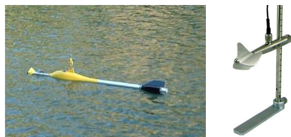
Figure 1: Current meter on the cableway (left side) and on the rod (right side) (Copyright: Seba Hydrometry)
