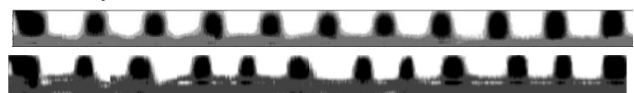
Figure 6: Vortex structure in annular gap for TVF Re = 126 (above) and with WVF Re=153 (below). Black = negative velocity, white = positive velocity, upper part = inner gap width, lower part = outer gap width
