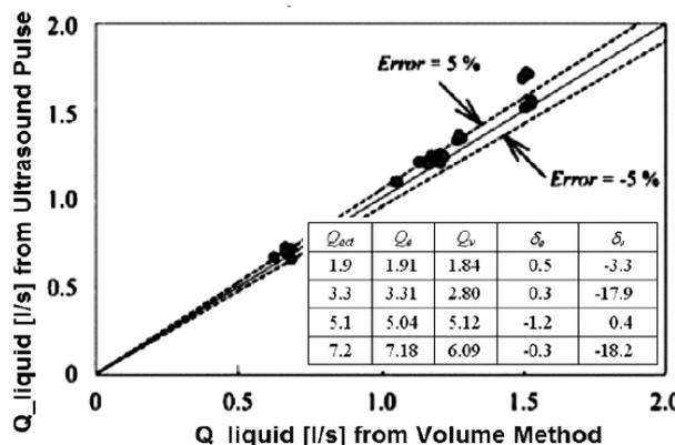
Fig. 12 Flowmetering accuracy for liquid volume flow rate
