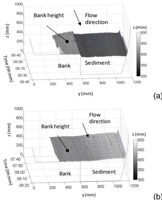
Figure 6: Temporal variation of sediment bathymetry, (a) 10/10/2013 and (b) 11/20/2013 measurements
