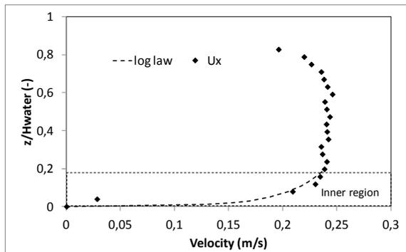
Figure 4: Longitudinal velocity profile and log law regression
