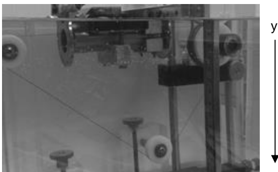
Figure 1: Doppler string phantom setup at SIK, Sweden.
