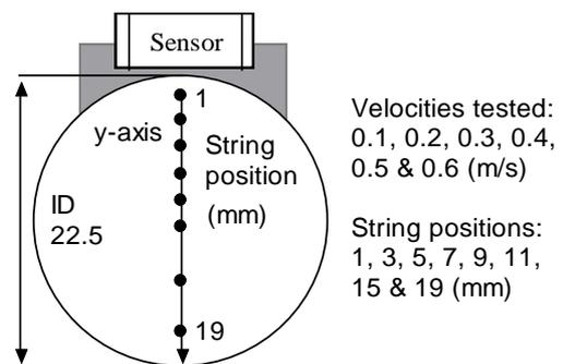
Figure 2: String positions and velocity range tested.
