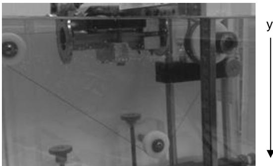
Figure 1: Doppler string phantom setup at SIK, Sweden.
