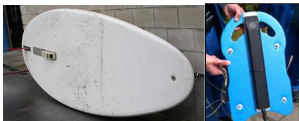
Figure 1: Installation of the two tested monitoring devices OCM Pro LR (on the left) and UB-Flow F156 below floats
