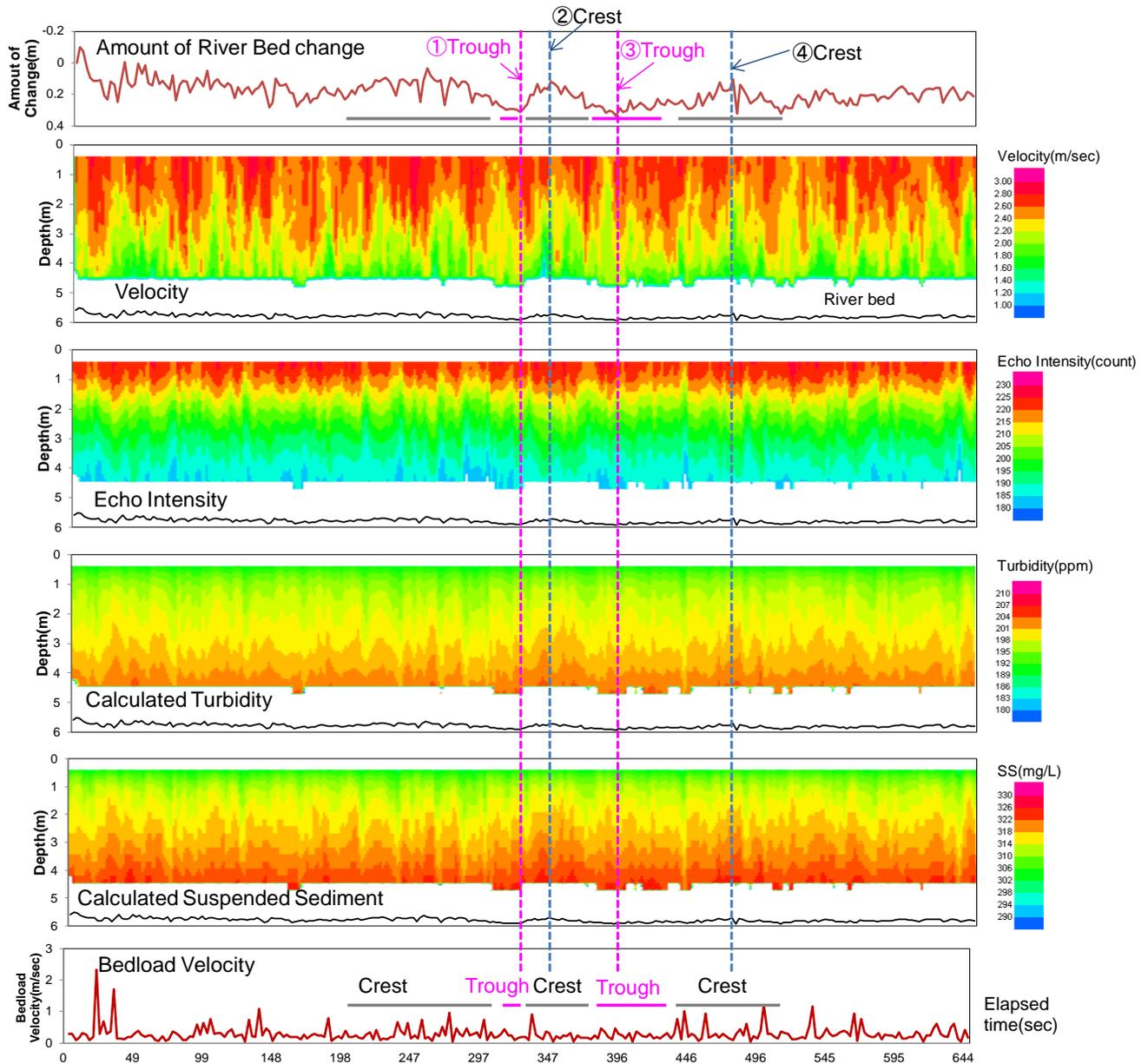
Figure 8: ADCP time series observation during flood
