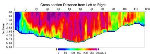
Figure 4 cross section velocity distribution
