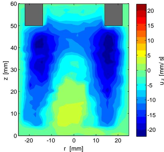
Figure 6: Flow field of DC current ( $I_{DC} = 48$  A) in the  $0^\circ$ -plane (at  $t = 7$  s, temporal resolution  $\Delta t = 143$  ms)
