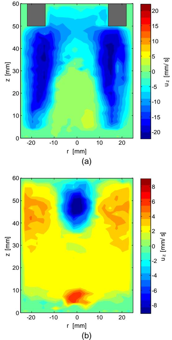
Figure 4: Flow field of electric pulse current (a) in the electrode plane ( $0^\circ$ -plane) and (b) in the plane between the electrodes ( $90^\circ$ -plane) (at  $t = 7$  s,  $I_{peak} = 151.8$  A,  $f_c = 50$  Hz,  $\tau = 0.1$ , temporal resolution  $\Delta t = 143$  ms)
