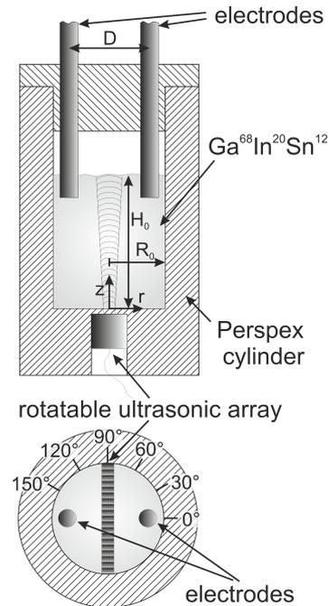
Figure 3: ECP setup with parallel electrodes
