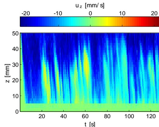
Figure 5: Spatio-temporal map of velocity profile below the electrode ( $r = -17$  mm in  $0^\circ$ -plane) of pulse current ( $I_{peak} = 151.8$  A,  $f_c = 50$  Hz,  $\tau = 0.1$ )
