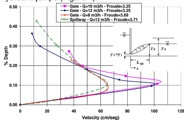
Figure 4: Velocity distributions in hydraulic jumps.
